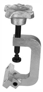
These unique C Clamps have a hinged pad for fastening permantently to a fixture, allowing them to swing clear for workpiece loading. The hinged mounting pad bolts to the fixture with two Socket-Head Cap Screws. Four-Prong Knob provides a firm grip for applications requiring quick tightening and high torque. Clamping screw is cast securely in the knob and has a removable swivel foot. Available in four sizes.
